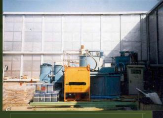
Lubrication & Backfill grouting Plant Muck pit
